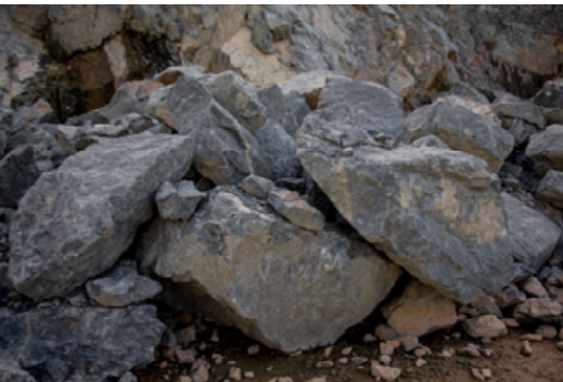
Left: 8 Ton Class riprap ( D_{50} size = 71").
