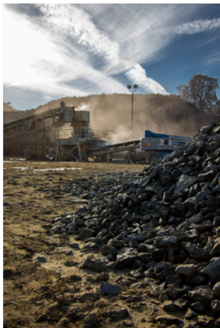
Light-class riprap (D 50 size = 18") at George Reed's Jackson Valley quarry.
