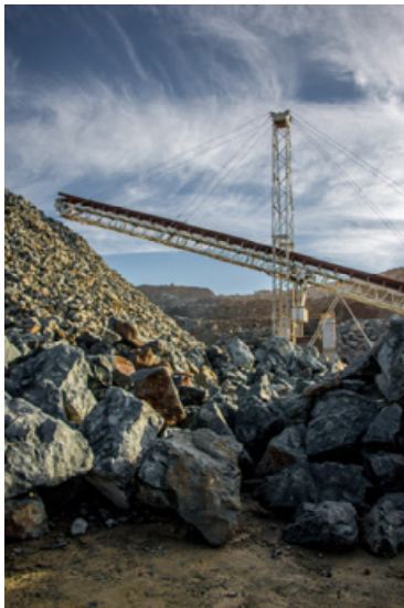
1 Ton Class riprap ( D_{50} size = 36") at George Reed's Jackson Valley quarry.
