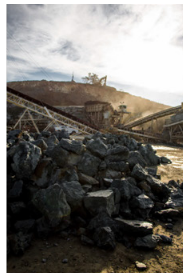
1/4 Ton Class riprap (D 50 size = 23") at George Reed's Jackson Valley quarry.
